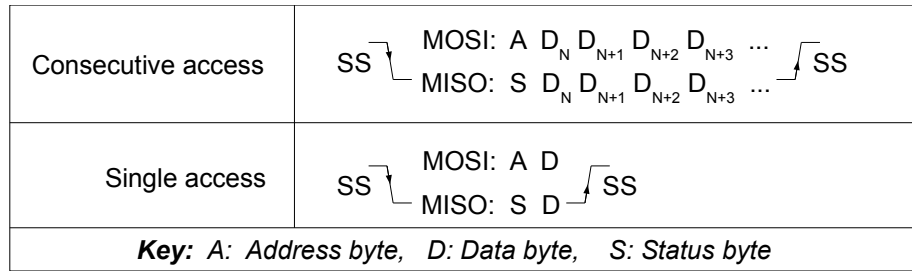
Fig. 7: Single byte and sequential byte accesses
